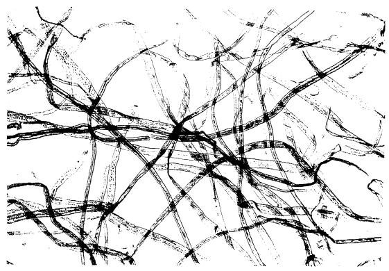
1. Isolated Longitudinal Tracheids from a Coniferous wood. <code>SOFTWOOD\_RIBBONS</code> Light micrograph.  $60 \times$
